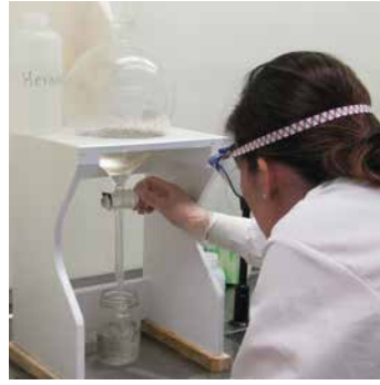
B) Remaining materials are funnelled through hexane and water to capture L2 larvae and remove sunken debris.
